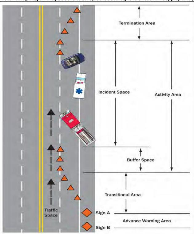
9. The following chart associated with MUTCD (Manual of Uniform Traffic Control Devices) TIMA (Traffic Incident Management Applications) Distances should be used as a guide for placement of cones and signs, should the circumstances allow.
